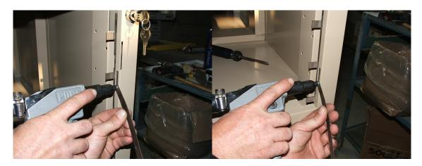
5. Insert the thumb latch into the thin, front slot of the cabinet and rivet the latch to the lock bar. The lock bar should slide up and down. Apply oil or other lubricant if needed.
